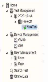
Three types of structures can be established under the test management node, which are folders, projects, and tests. By adding, deleting, copying, pasting and other operations, the hierarchical, efficient and orderly management of projects and tests can be realized.
